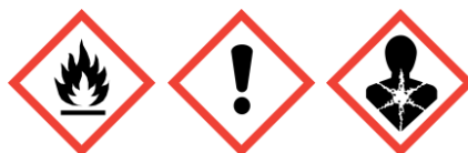
Flame Exclamation mark Health hazard
